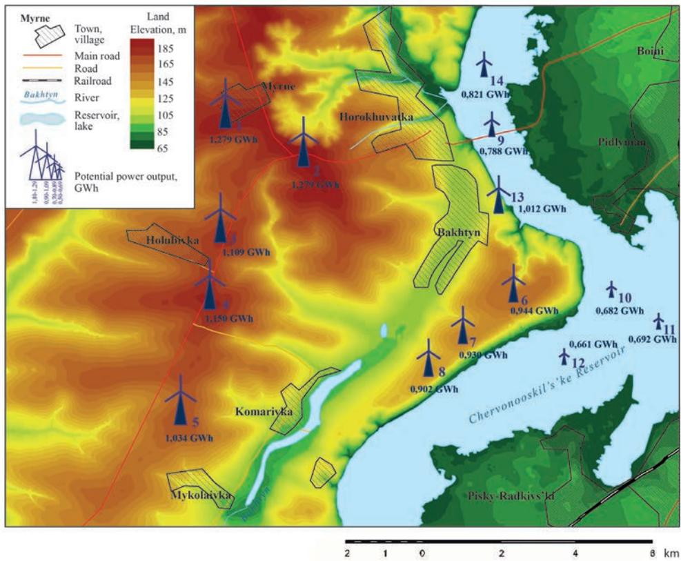
Fig. 2. Calculated output power and potential locations of wind turbines within the research area
